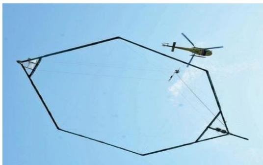
*The aquifer mapping survey will help identify zones for drilling productive French wells to meet the city's water demand*
